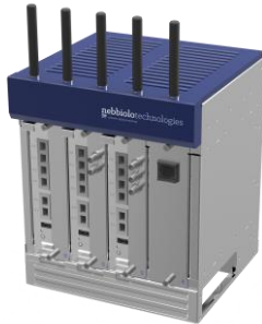
Figure 3-4. A prototype of an edge node by Nebbiolo Systems/TTTech.
