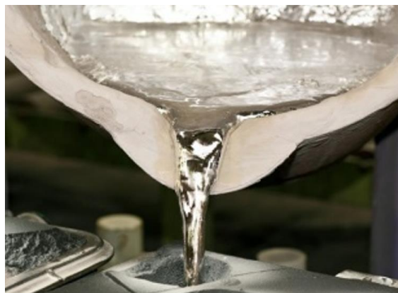
Figure 2-1: Filling aluminium into a sand mould
